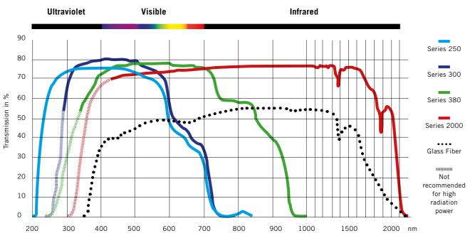
Measured with 2α=50° (Series 250 2α=34°), length 2000mm, active core Ø5mm
